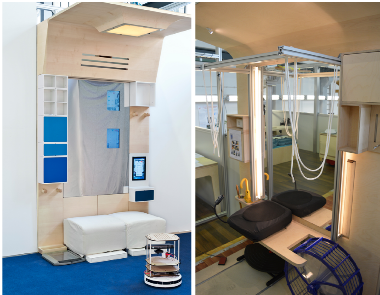
Figure 1.4 / The entrance module; Left: the result of the first LISA project; Right: the designed improved version, with novel assistive functions. As depicted, the original design from the first LISA project has been improved, so that less space for this terminal is now consumed.
