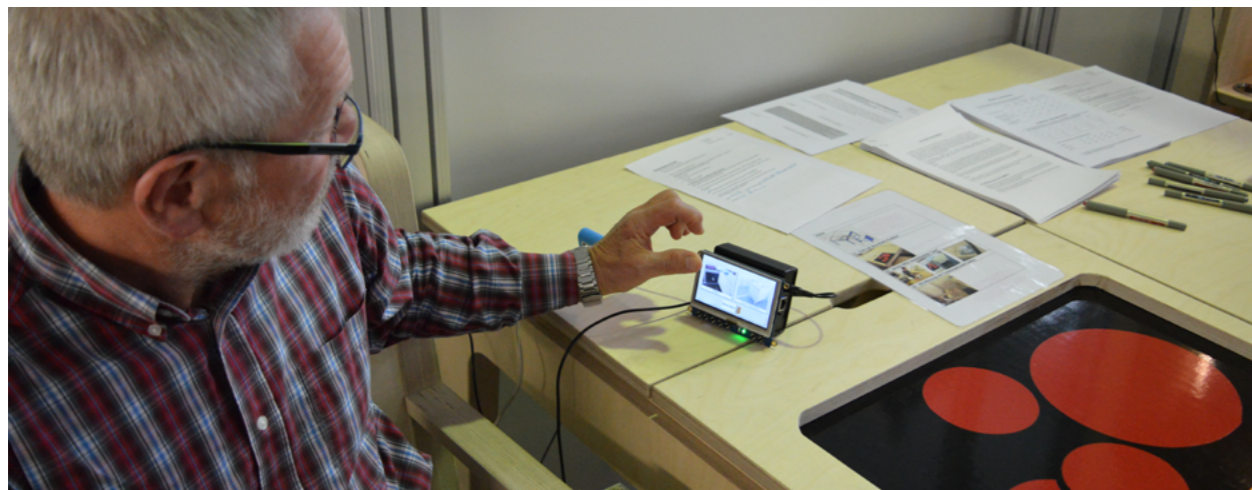
Figure 2.11 / The capacitive electrodes modular, attached to the sides of the armrests of a test chair with the controlling touchscreen for the table.
