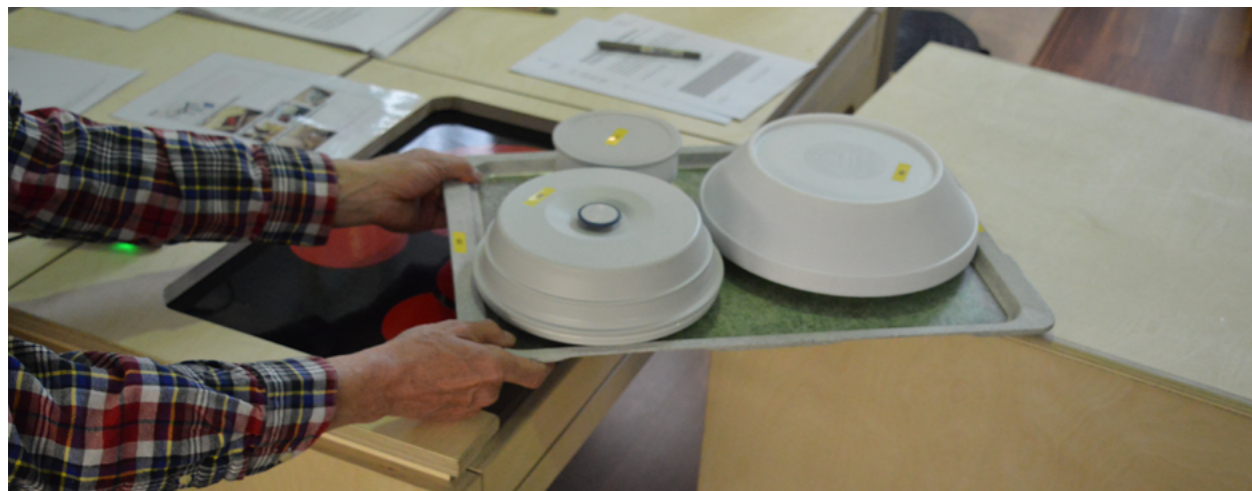
Figure 2.10 / Food terminal module with a mobile platform hidden in a table. It can autonomously drive and be controlled by a touchscreen, which is placed on the table.
