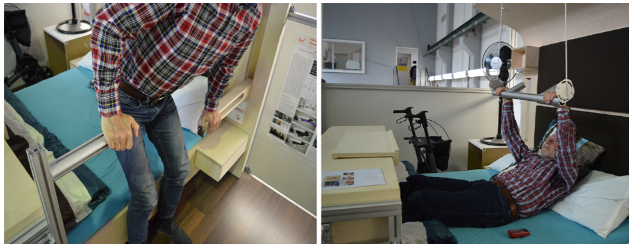
Figure 2.14 / Left: the unobtrusive implemented handles. Right: the remote-controlled handle. Left bottom: the integrated table on a sliding rail, which was unfolded in the figure at the right bottom.
