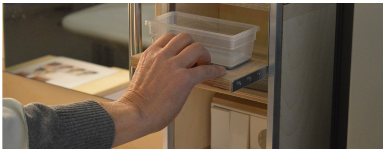
Figure 2.8 / Testing the mock-up cabinet lift system.
